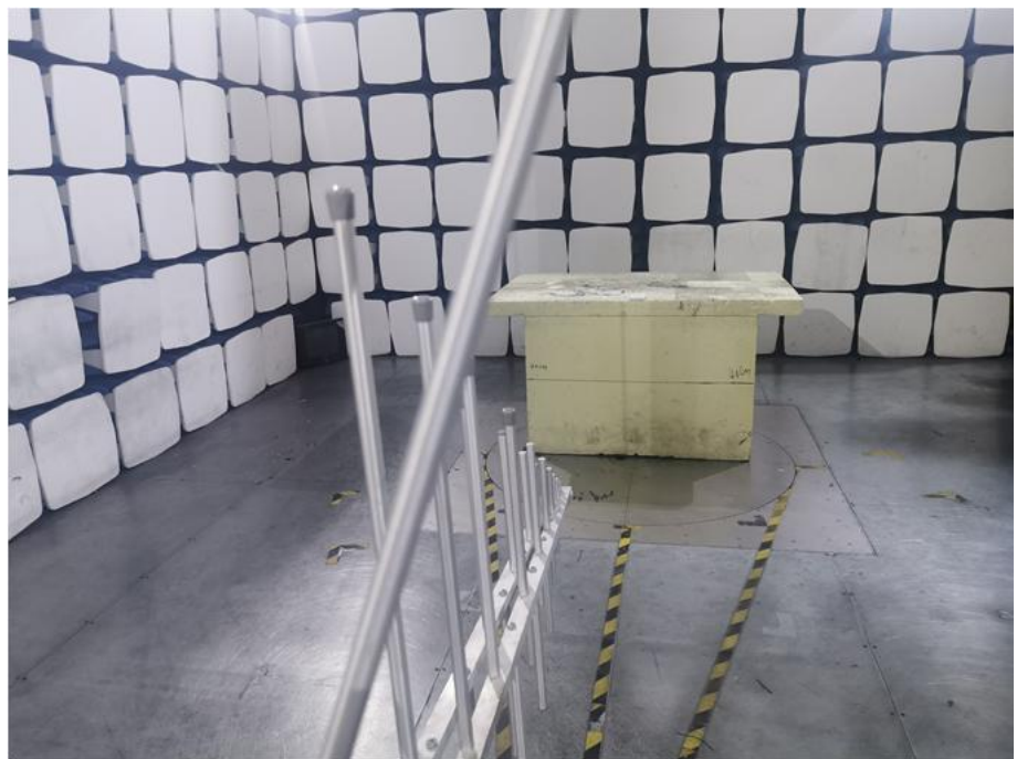
Radiation Emission Test Setup (30MHz to 1GHz)
