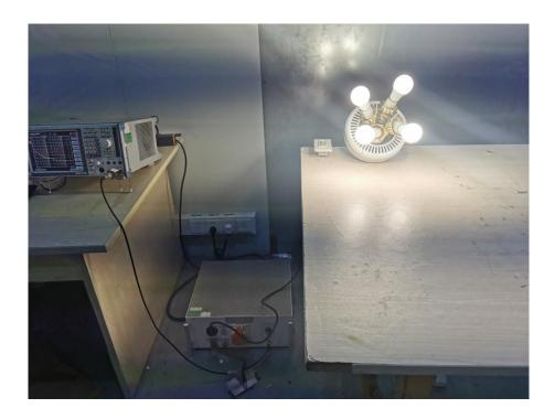
Radiation Emission Test Setup (Below 30MHz)
