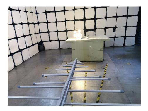
Radiation Emission Test Setup (1GHz to 18GHz)
