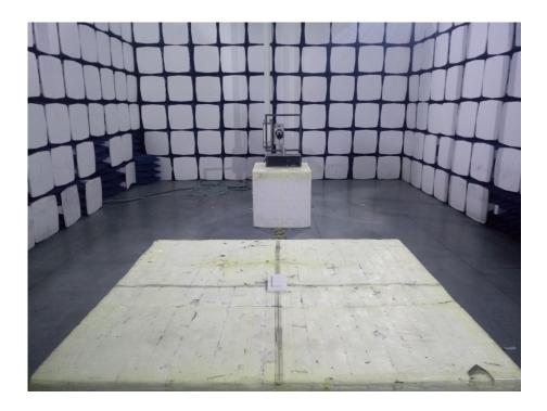
Radiation Emission Test Setup (30MHz to 1GHz)
