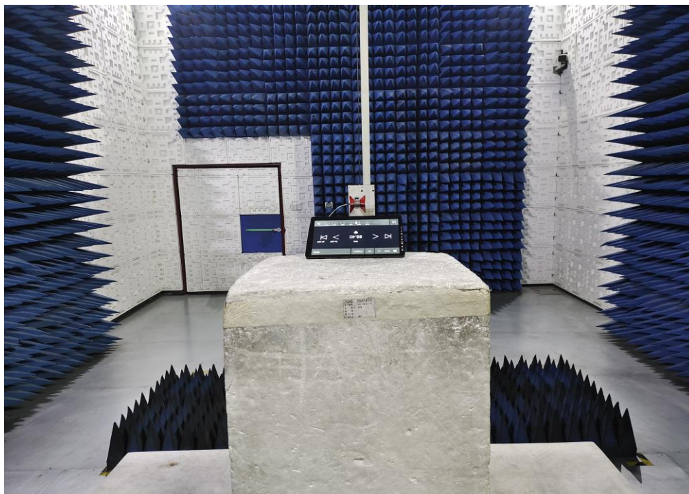
RADIATED EMISSION TEST SETUP ABOVE 1GHz
