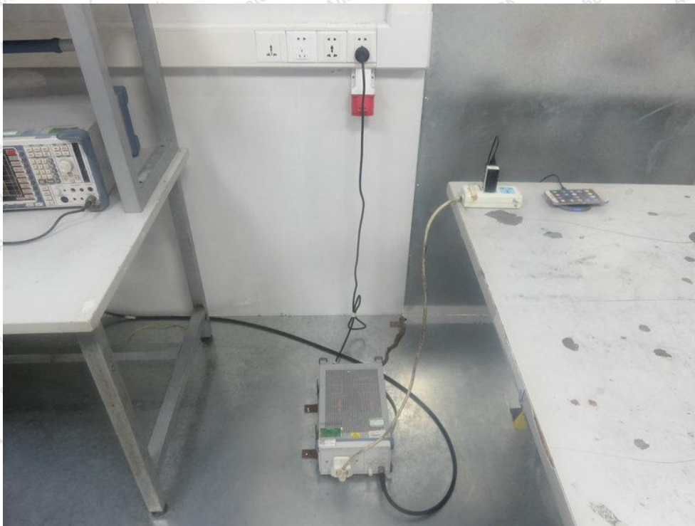
Photo of Conducted Emission Measurement
