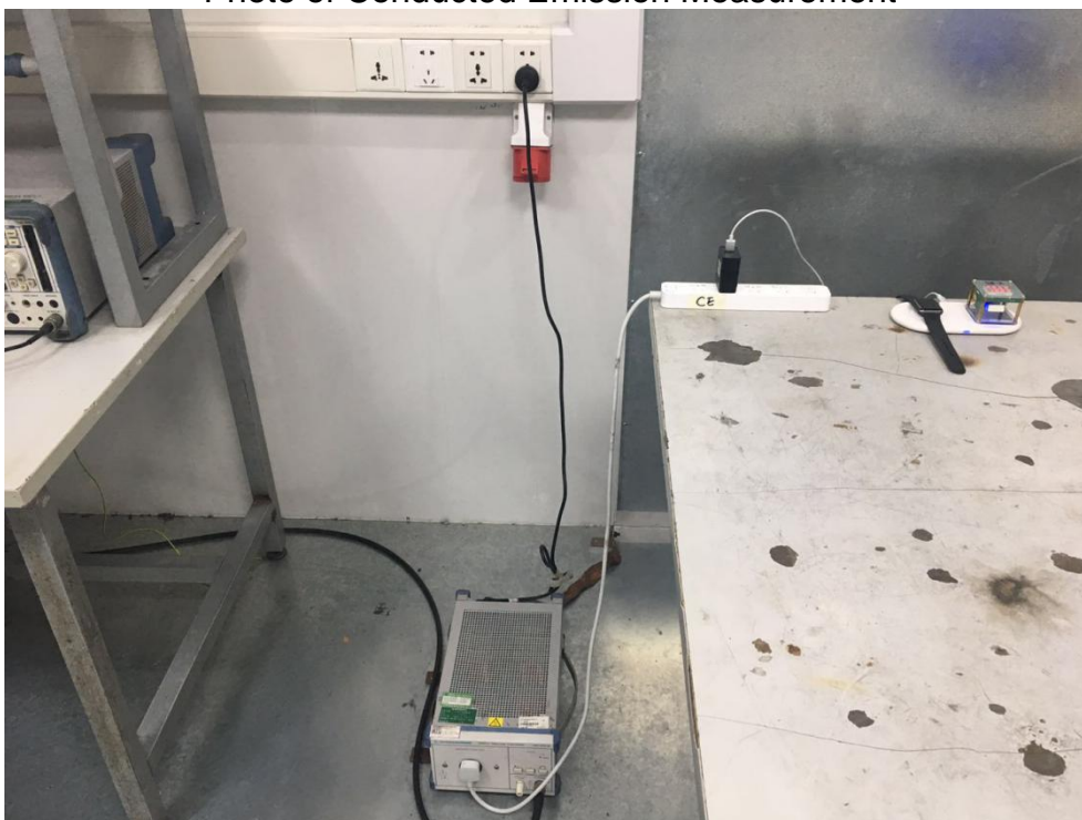
Photo of Conducted Emission Measurement
