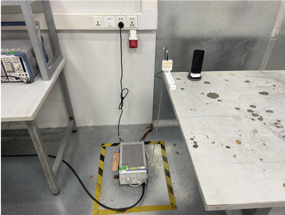
Photo of Conducted Emission Measurement
