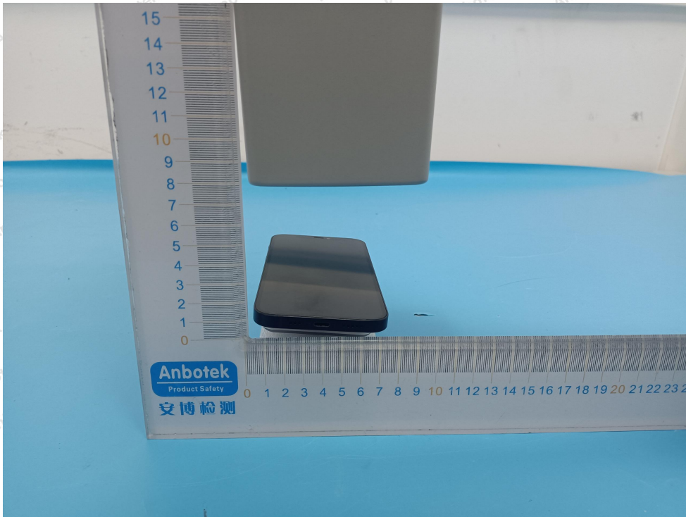
Photo of MPE Measurement at 6 cm
