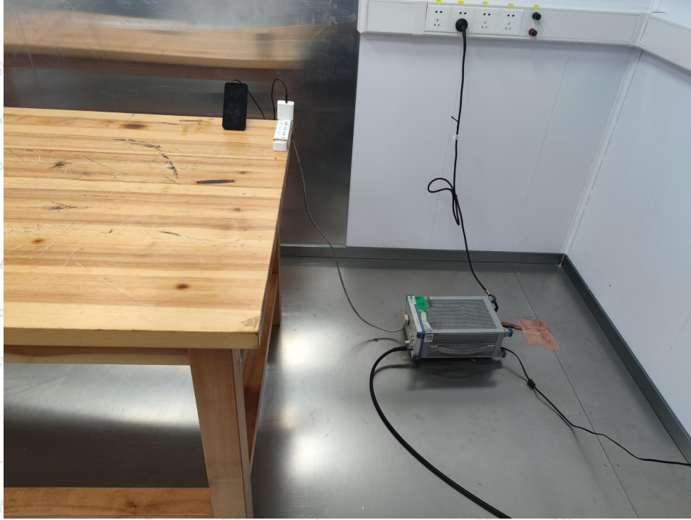
Photo of Conducted Emission Measurement
