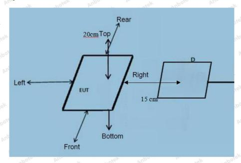
Note: Measurements should be made at 15 cm surrounding the EUT and 20cm above the top surface of the EUT.
