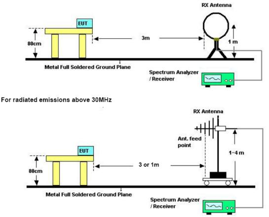
Above 10 GHz shall be extrapolated to the specified distance using an extrapolation factor of 20 dB/decade from 3m to 1m.
