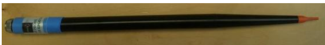
Figure-MVG COMOSAR Dosimetric E field Dipole
