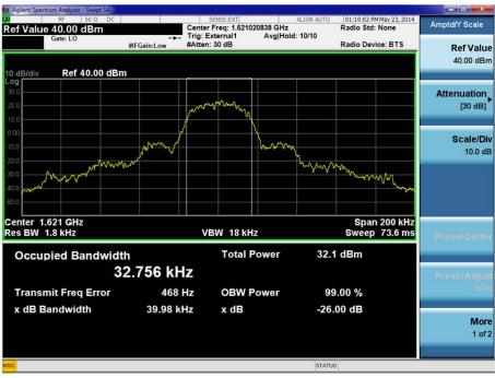
Traffic, broadcast, and ring alert channels use differentially encoded quaternary phase shift keyed (DE-QPSK) modulation with 40% square root raised cosine pulse shaping. The burst transmission rate is 25ksps or 50 kbps. The phase of the QPSK symbol states relative to the carrier phase is (Symbol State/Phase in deg): 00/0, 01/-90, 10/+90, 11/180.
