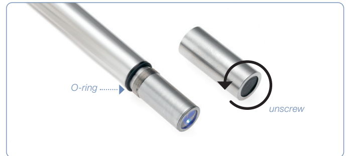
Figure 12: Replacing the ODO cap
