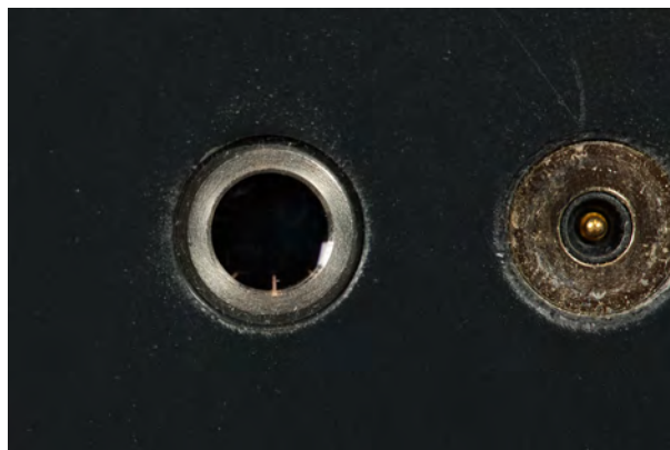
Fig. 55: Optical Channel at the Bottom of the Mobile Device.
