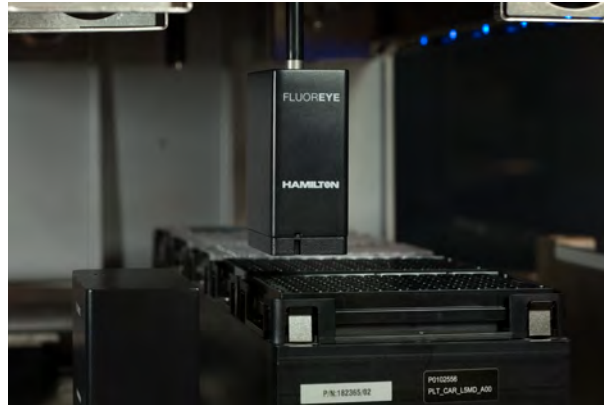
Fig. 9: Mobile Device Measuring the Fluorescence
