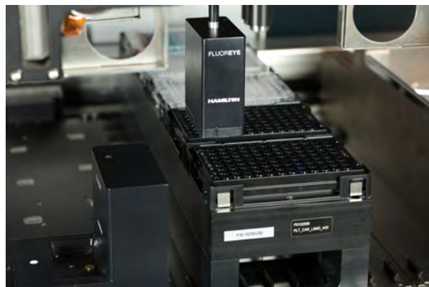
Fig. 13: Measuring Distance Between Liquid Surface and Lower Border
