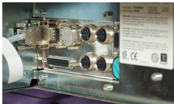
Fig. 23: Periphery Connector at the Left Side of the Instrument
