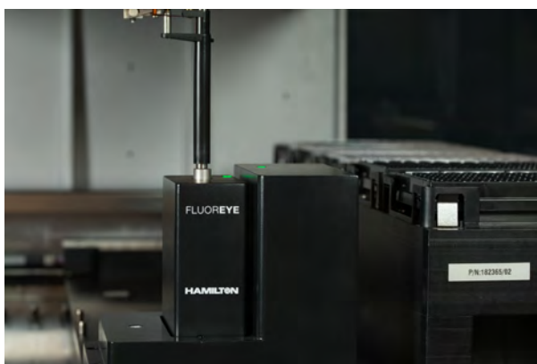
Fig. 8: 1000ul Pipetting Channel Picking Up the Mobile Device
