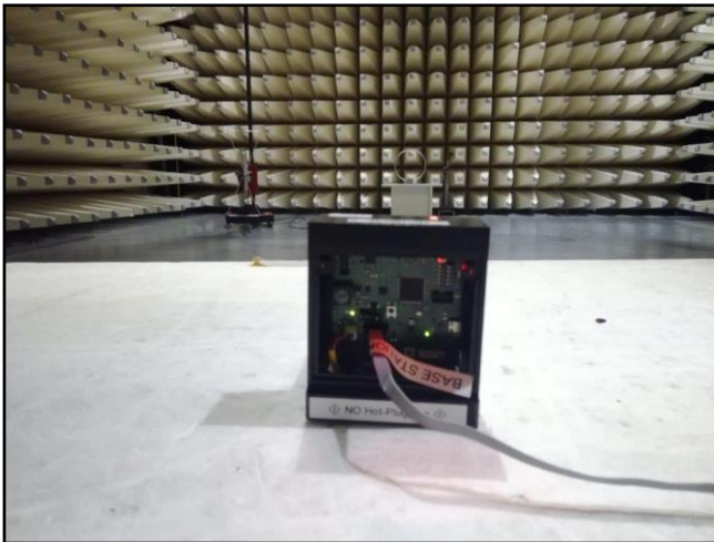
Loop-Antenna: EMCO 6502A (Correction factor @ 13.56MHz +9.5 dB)
