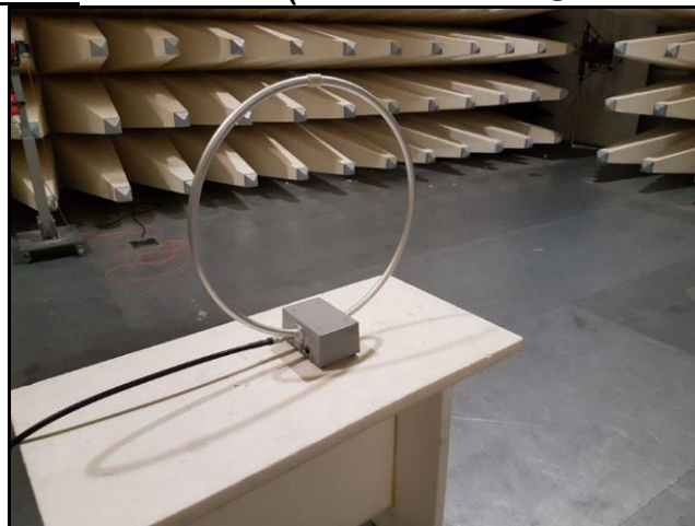
Loop-Antenna: EMCO 6502A (Correction factor @ 13.56MHz +9.5 dB)
