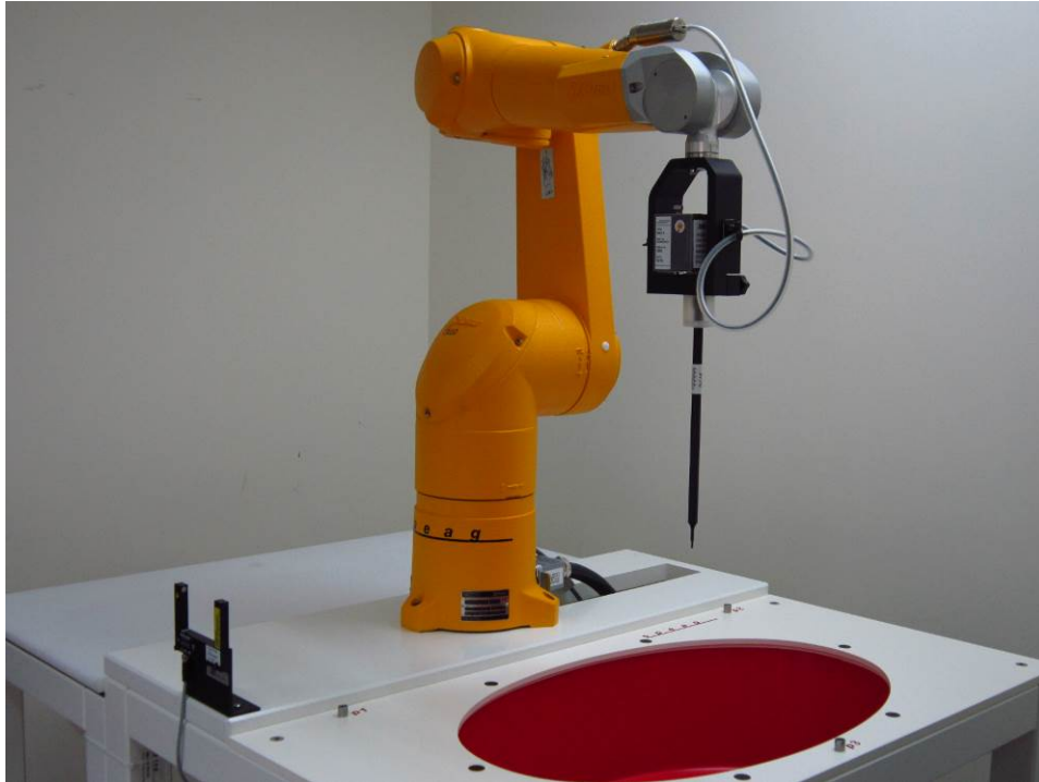
Fig.1 Photograph of the SAR measurement system
