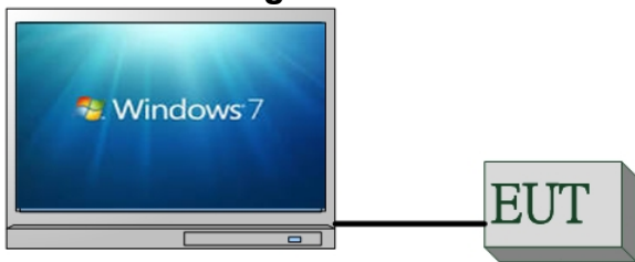
Fig. 2-2 Conducted (Antenna Port) Emission Configuration
