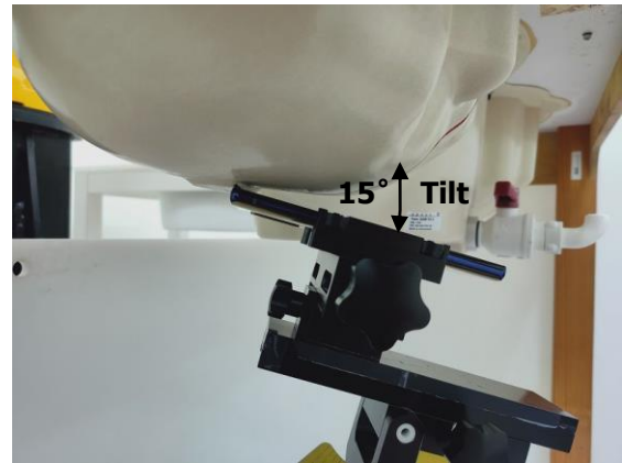
Fig.4 Right Head Section / Ear-Tilt Position(15°)
