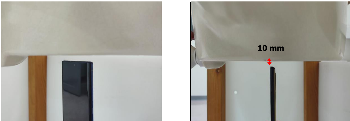
Fig.14 EUT Top side to flat phantom
