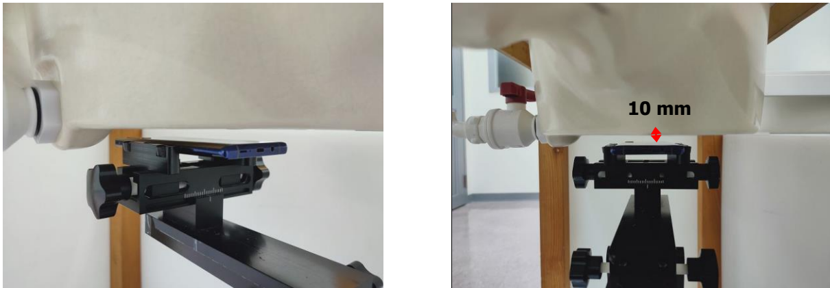
Fig.8 EUT Back side to flat phantom
