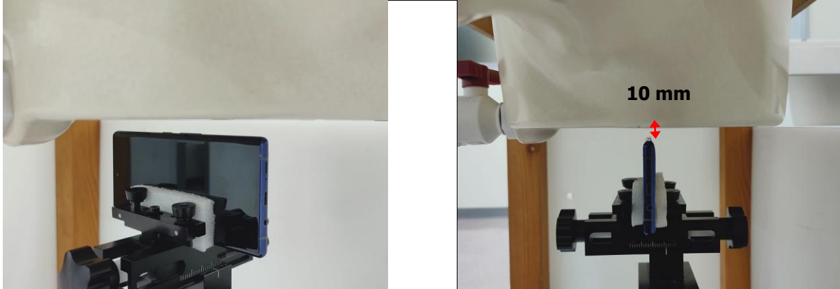
Fig.12 EUT Right side to flat phantom
