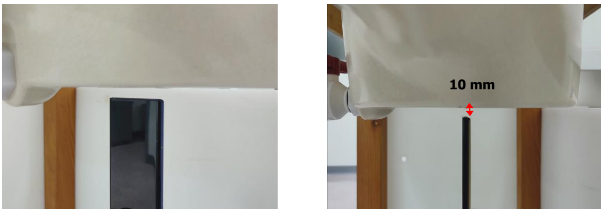
Fig.11 EUT Bottom side to flat phantom
