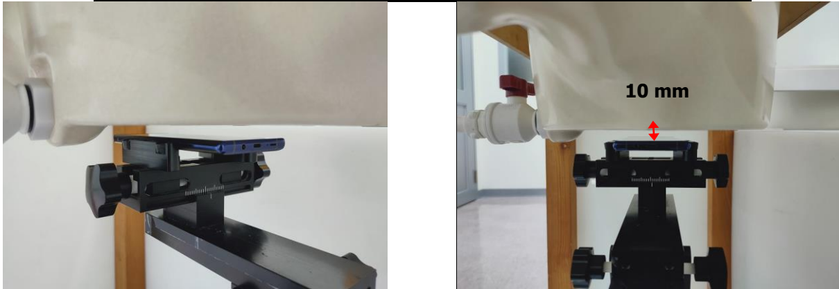
Fig.9 EUT Front side to flat phantom
