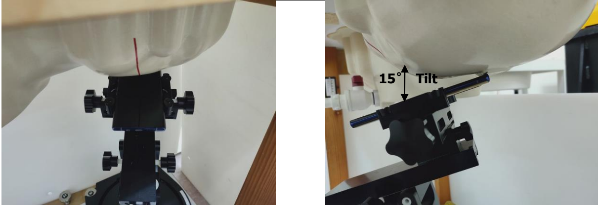
Fig.6 Left Head Section / Ear-Tilt Position(15°)
