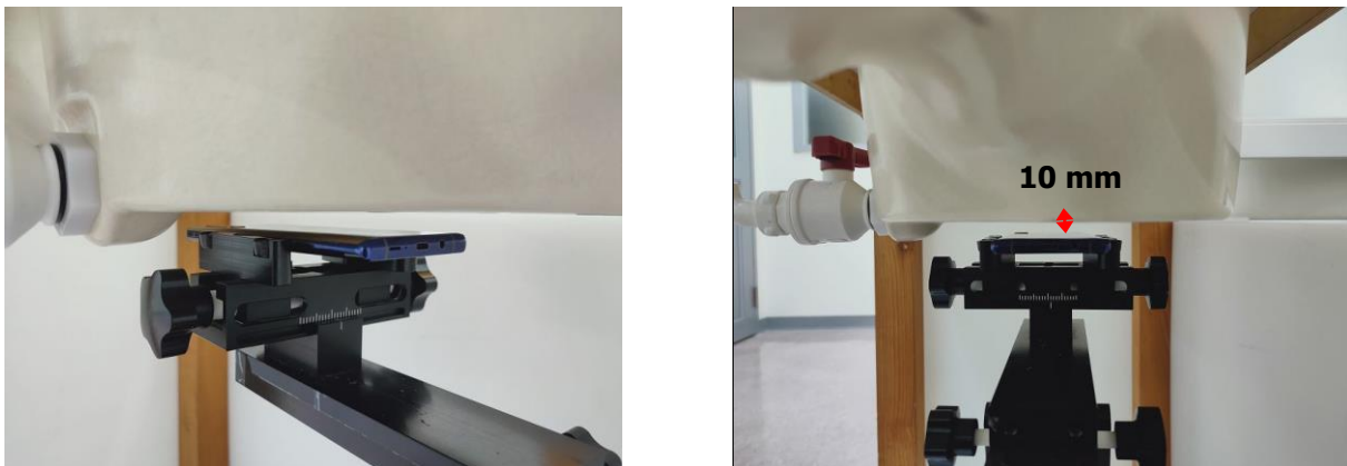
Fig.10 EUT Back side to flat phantom
