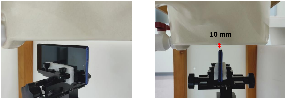
Fig.13 EUT Left side to flat phantom
