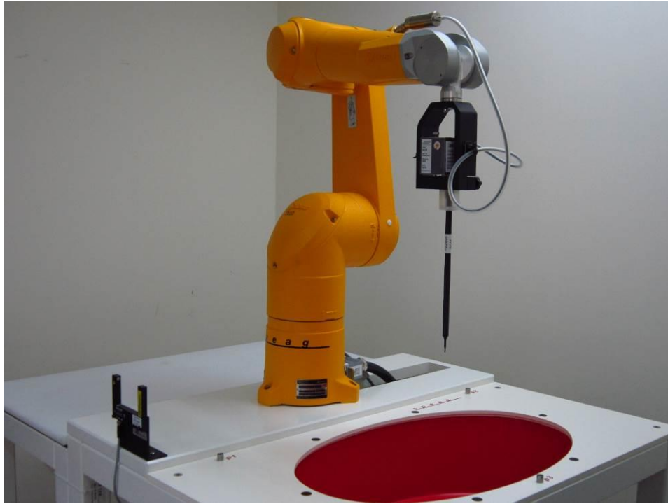
Fig.1 Photograph of the SAR measurement system
