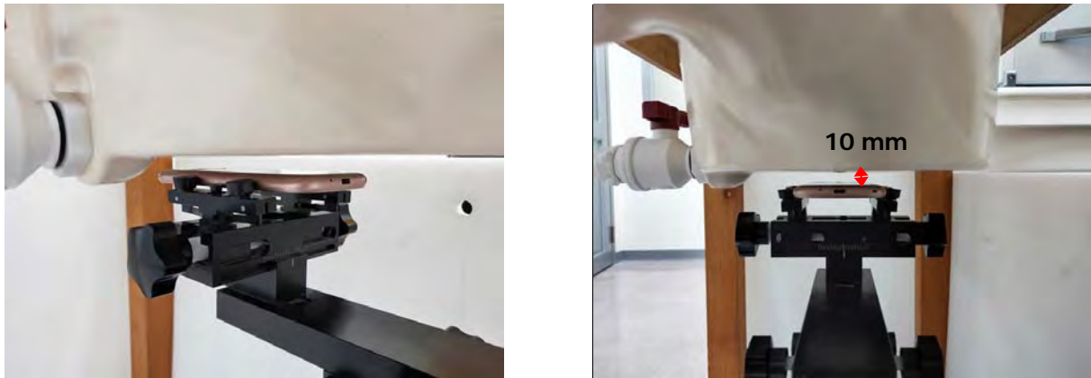
Fig.8 EUT Back side to flat phantom
