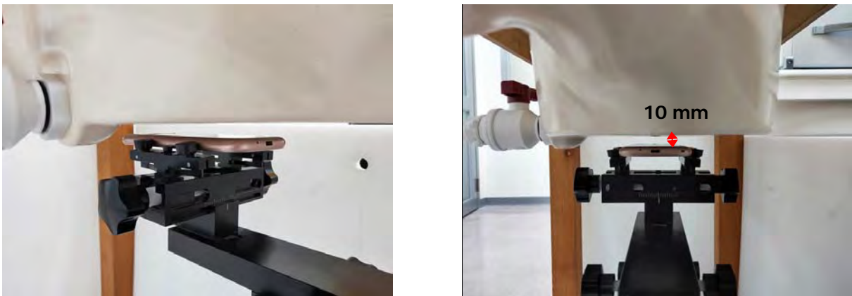
Fig.10 EUT Back side to flat phantom
