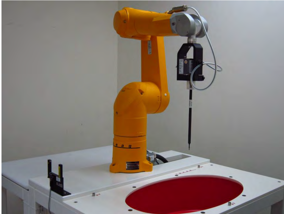
Fig.1 Photograph of the SAR measurement system
