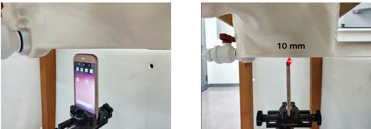
Fig.11 EUT Bottom side to flat phantom
