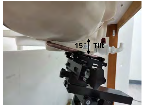
Fig.4 Right Head Section / Ear-Tilt Position(15°)
