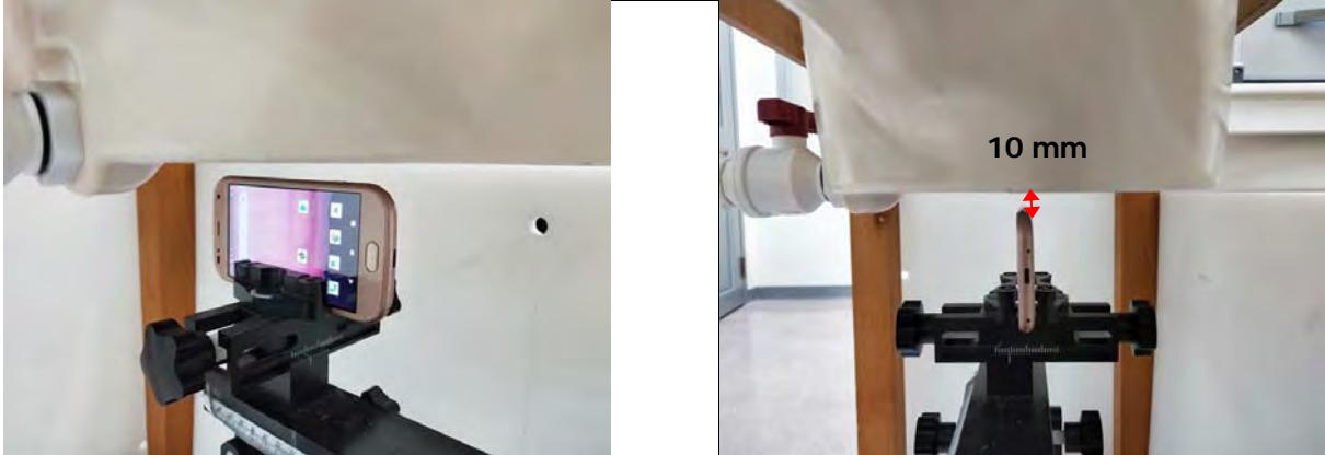
Fig.12 EUT Right side to flat phantom
