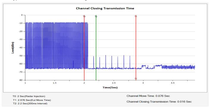
Verdict: Note: narrowing the sweep time as the good engineering process for the verification of transmission closing in 200ms
