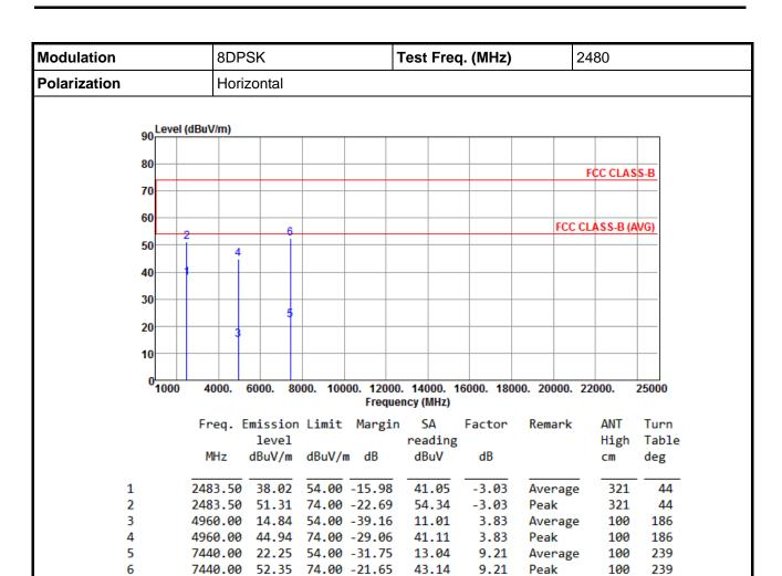
Note 1: Emission Level (dBuV/m) = SA Reading (dBuV/m) + Factor\* (dB) \*Factor includes antenna factor , cable loss and amplifier gain
