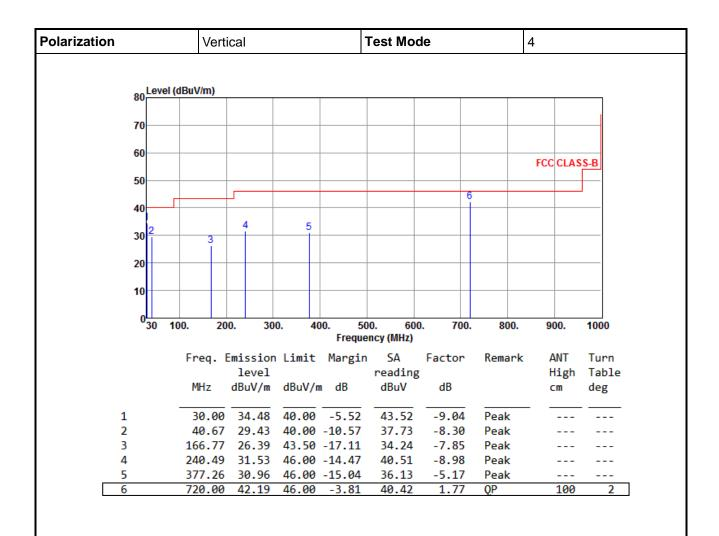
Note 1: Emission level (dBuV/m) = SA reading (dBuV) + Factor (dB)
