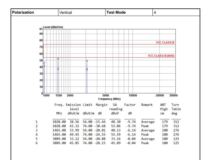
Note 1: Emission level (dBuV/m) = SA reading (dBuV) + Factor (dB)
