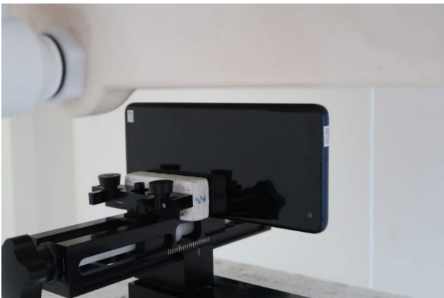
Left Side, Test Separation 10 mm
