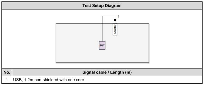
Note: The support notebook is disconnected from EUT and removed from test table after sending command to EUT to control EUT to transmit continuously.
