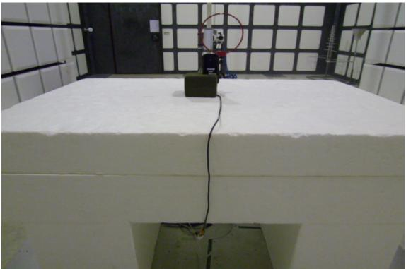
Radiated Emission Setup Photos (30MHz~1GHz)
