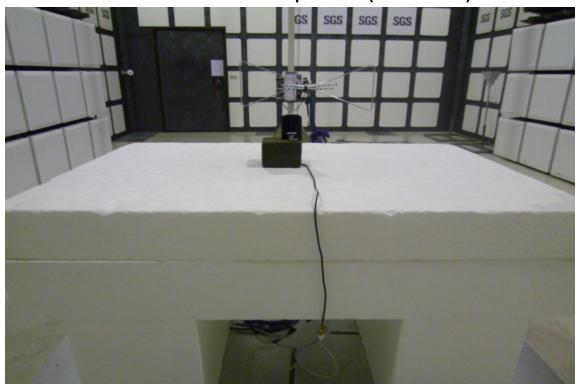
Radiated Emission Set up Photos (Above 1GHz)
