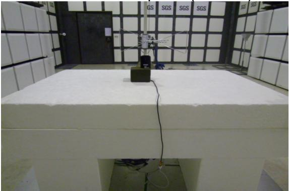
Radiated Emission Set up Photos (Above 1GHz)
