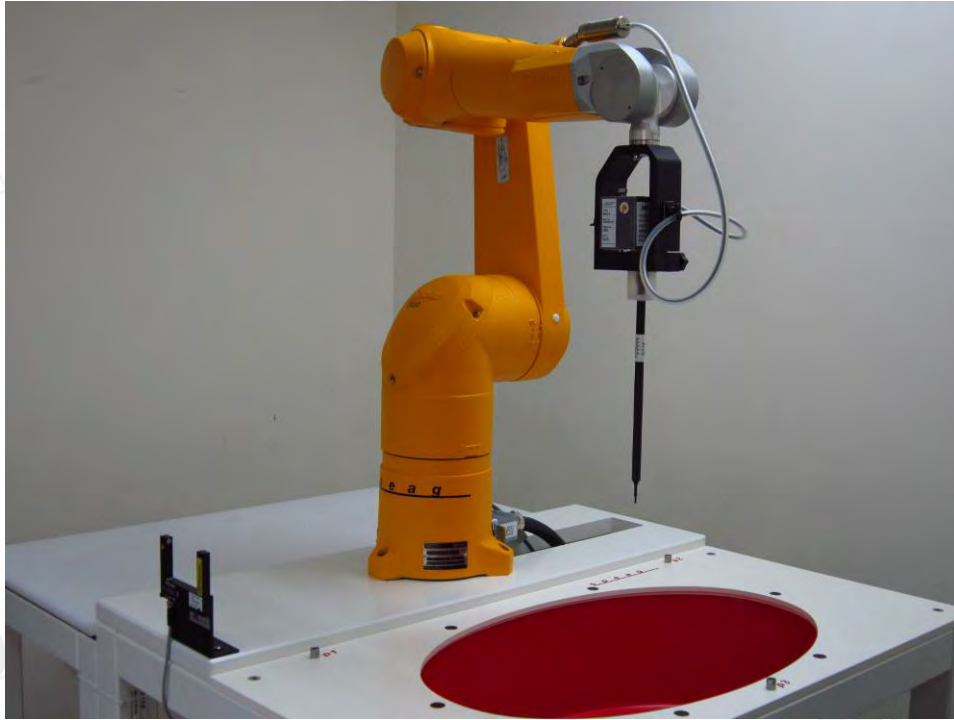
Fig.1 Photograph of the SAR measurement system
