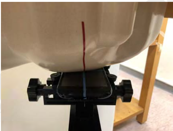
Fig.5 Left Head Section / Cheek-Touch Position
