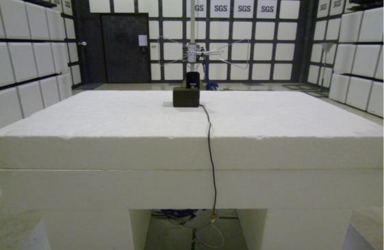
Radiated Emission Set up Photos (Above 1GHz)
