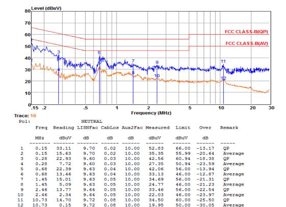
Remarks: 1. Measured = Reading + LISNFac + Cable Loss + Aux2 Fac. The emission levels that are 20dB below the official limit are not reported.
