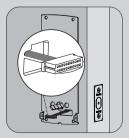
7. Attach cable assembly to the interior assembly PCB by lining up notches on top of cable connector to slots on PCB
