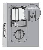
If the reset is successful, the latch bolt will extend on its own to learn the handing orientation of the door.
