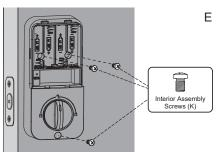
Test the lock by rotating the thumb turn to see if the bolt can be extended and retracted smoothly.
