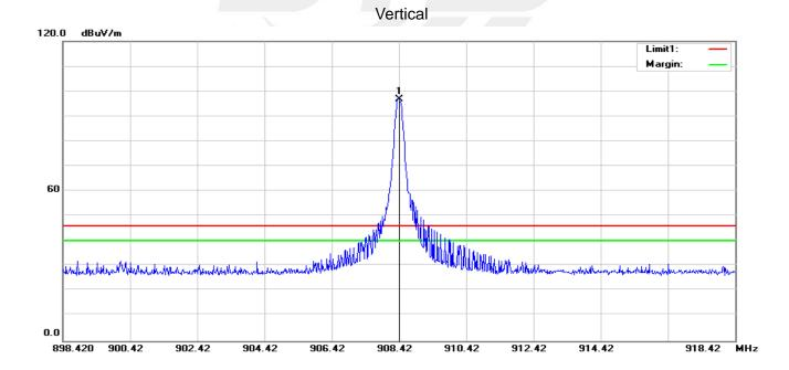
No. Frequency Reading Correct **Duty cycle** Result Limit Margin Remark (MHz) (dBuV) Factor(dB/m) Factor(dB/m) (dBuV/m) (dBuV/m) (dB) 908.4200 1 97.08 -0.22 96.86 114.00 -17.14 Peak -2 908.4200 -0.22 97.08 -11.63 85.23 94.00 -8.77 AVG
