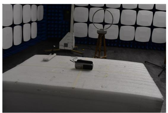
3. Radiated emission (9KHz-30MHz)
