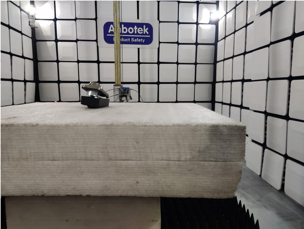
Photo of Radiation Emission Test (above 1GHz)
