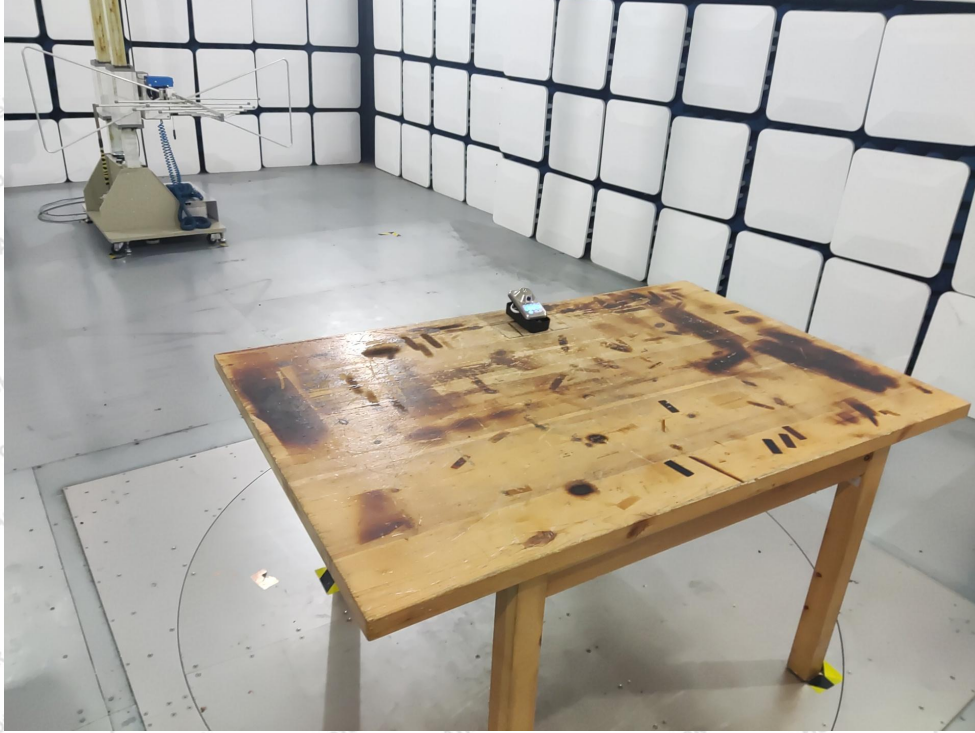
Photo of Radiation Emission Test (below 1GHz)
