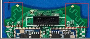
The antenna is PCB antenna. ANT1/ANT2 gain is 0 dBi.
