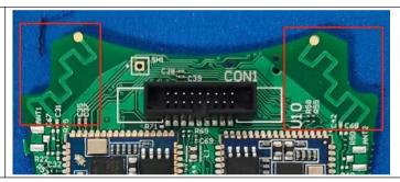
The antenna is PCB antenna. ANT1/ANT2 gain is 0dBi.
