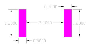
**♦ 2<sup>nd</sup> Layout Dimensions in Clearance area**(Size=8.0\*3.0mm)
