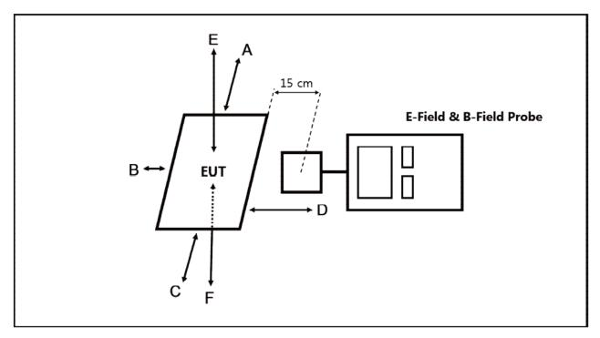
Note: Measurements should be made from all sides and the top of the primary/client pair, with the 10cm measured from the center of the probe(s) to the edge of the device.
