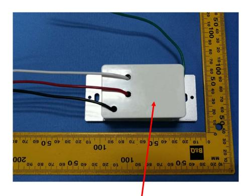
For Control of permanently installed incandescent, halogen lamp fixtures only. For supply connection, use wires rated for at least 75  $^{\circ}$ C.
