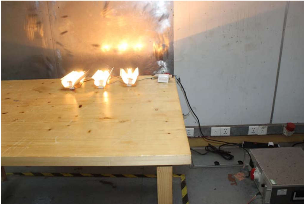
Photograph of set-up for ac power line Conducted emission
