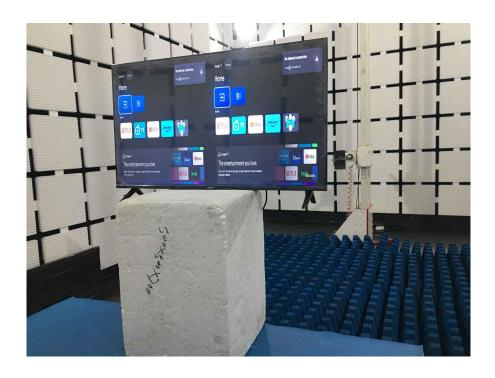
Conducted Emissions at AC Power Line (150kHz-30MHz)
