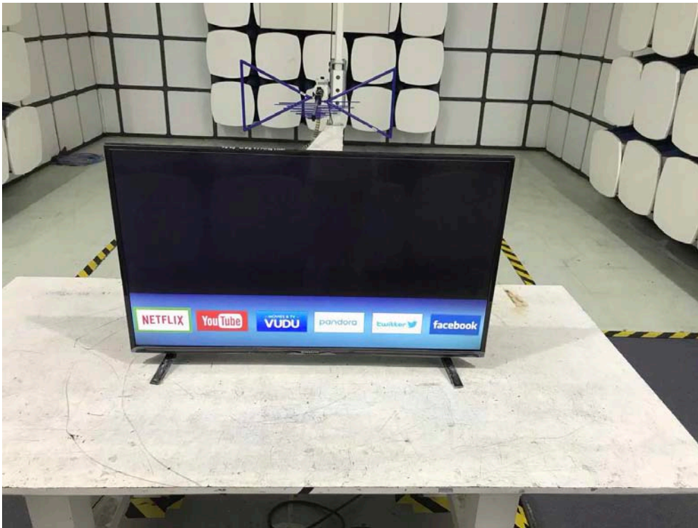
Radiated Test (30-1000 MHz)
