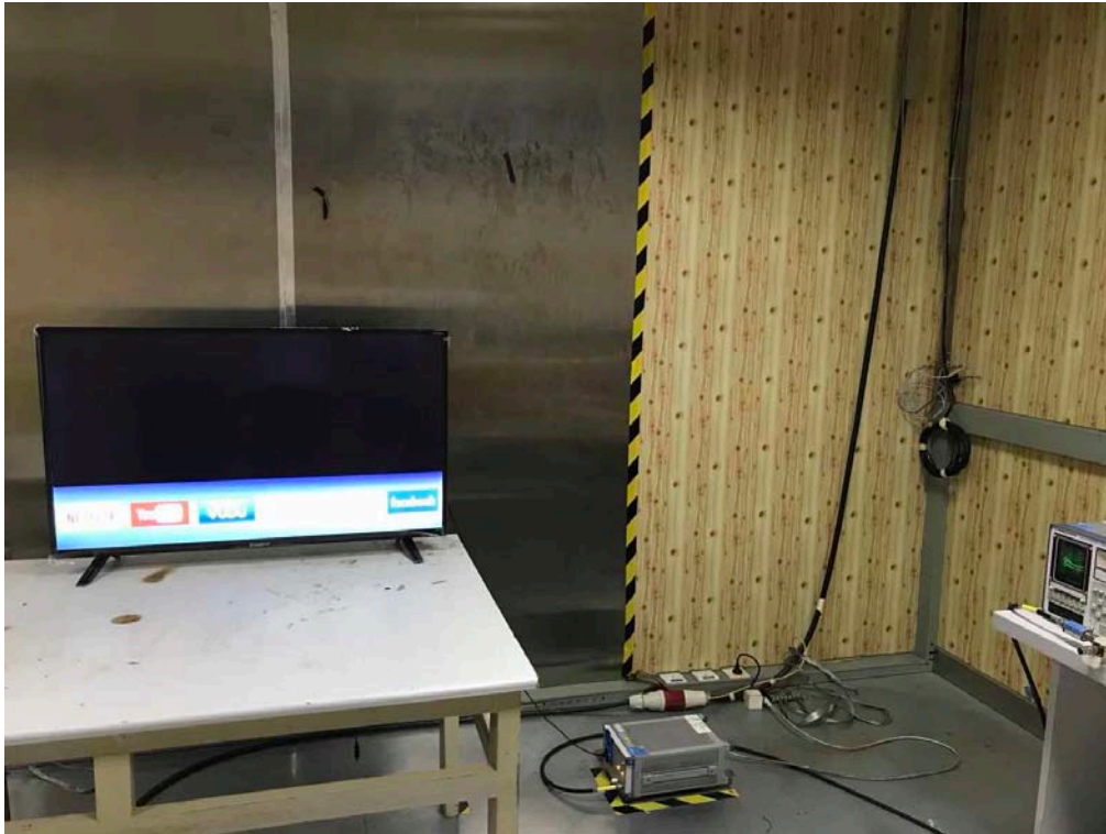
Conducted Test (0.15-30 MHz)
