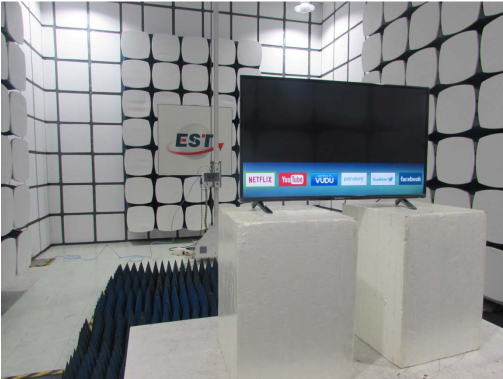
Radiated Test (Above 1000 MHz)
