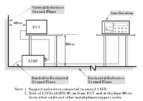
The setup of EUT is according with per ANSI C63.4-2014 measurement procedure. The specification used was with the FCC Part 15 B Class B limits.
