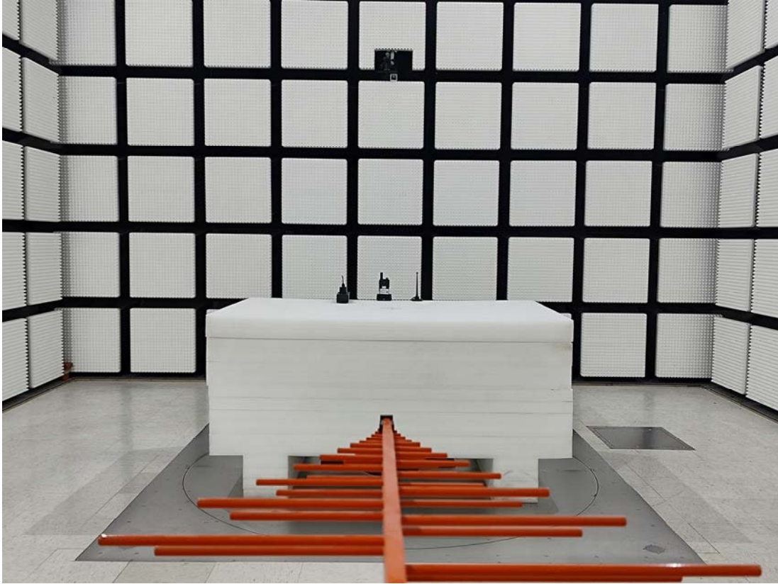
Radiated Emission Below 1GHz Rear View
