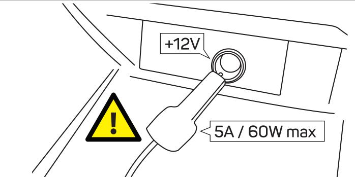
**ATTENTION!** After installation, devices/consumers with more than **5A / 60W** shall not be operated on the +12V socket. Otherwise a risk of overvoltage can occur!
