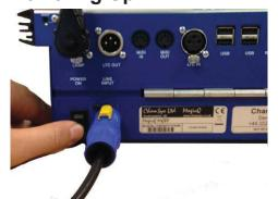
To power up the console press the power switch on the back panel. The blue LEDs around the left and right of the display should light, after a few seconds the screen will come to life and you will see the operating system loading.
