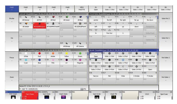
For indexed attributes such as colour wheels and gobo wheels, the button associated with each encoder can be used to bump the attribute value to the next range. Pressing SHIFT and the button bumps back to the previous range.
