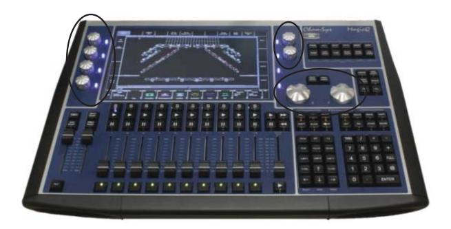
The function of the rotary encoders also changes according to the active window with the current function being displayed adjacent to the encoder.
