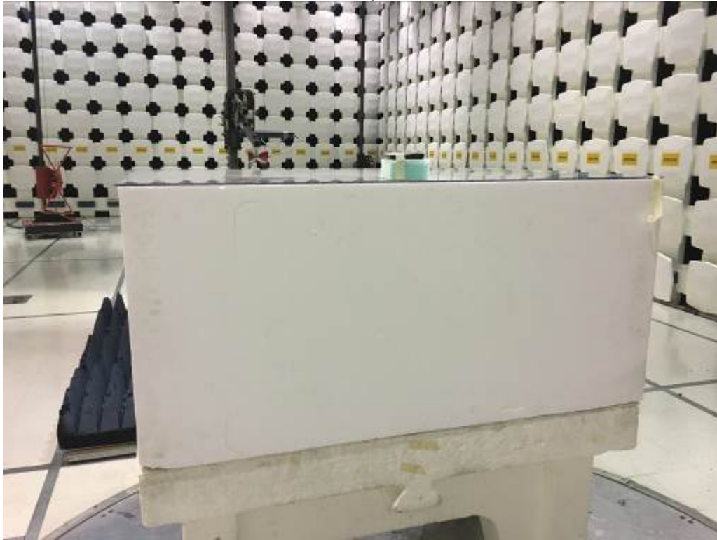
Radiated Setup, 1-18 GHz
