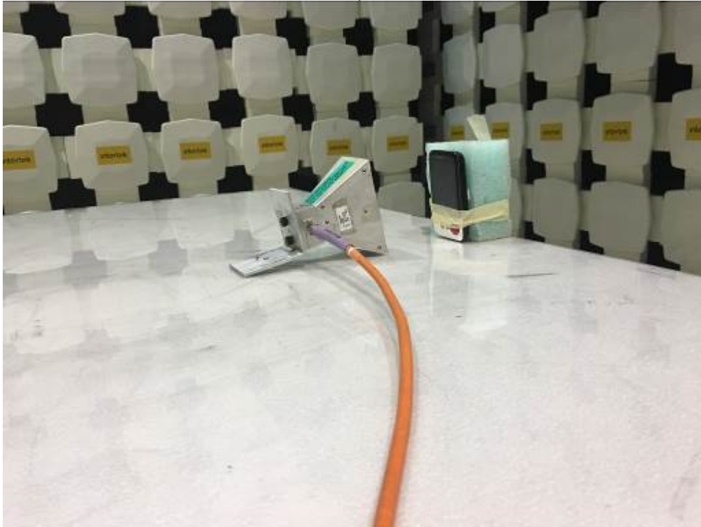
Radiated Setup, 18-25 GHz
