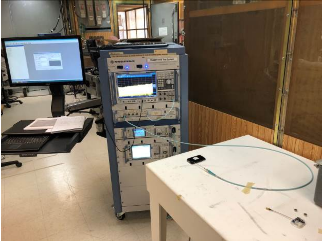
Antenna Port Conducted Test Setup
