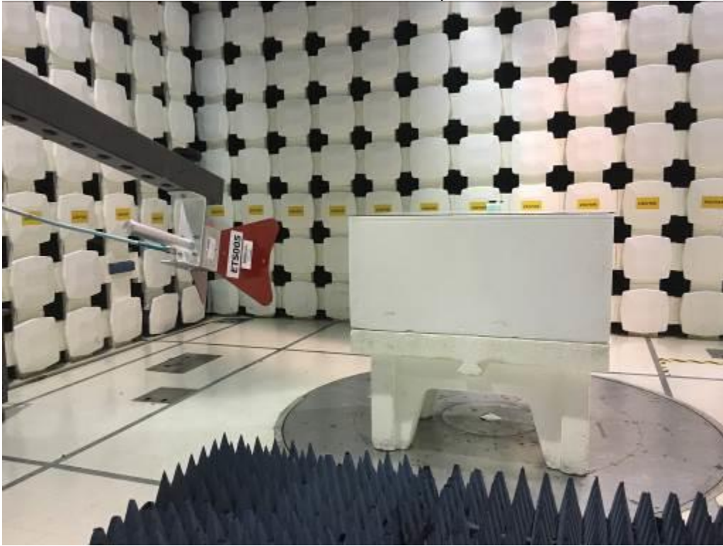
Radiated Test Setup
